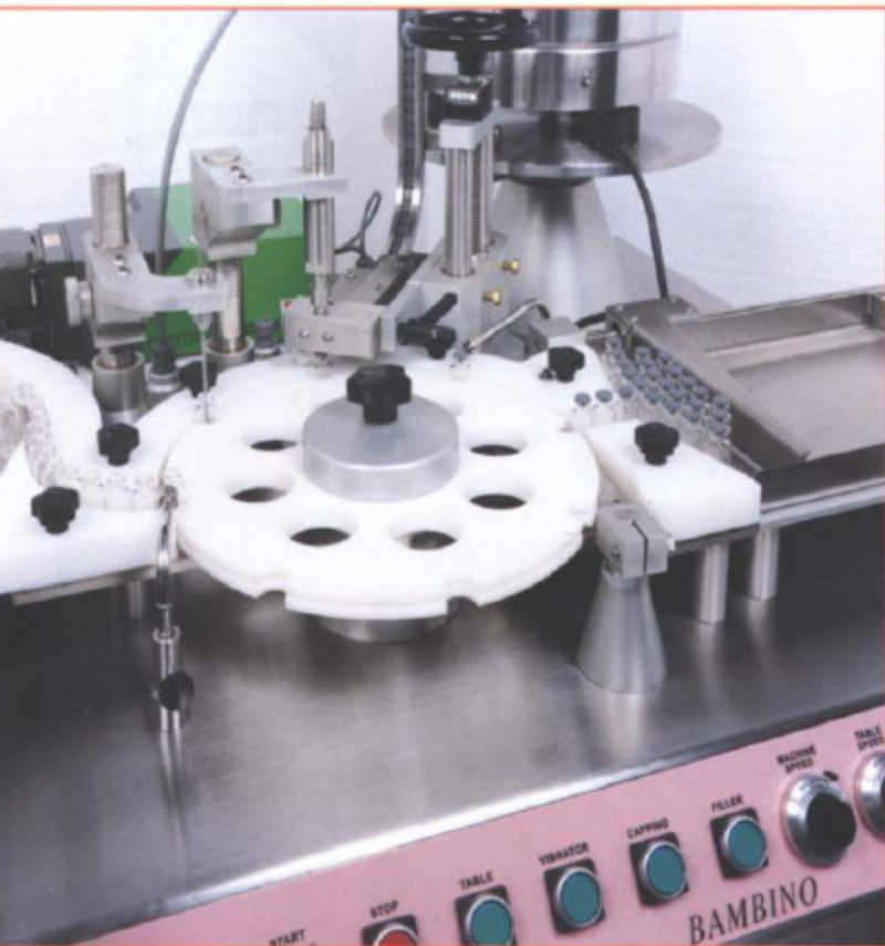
◀ Bambino FS with filling and stoppering stations.
