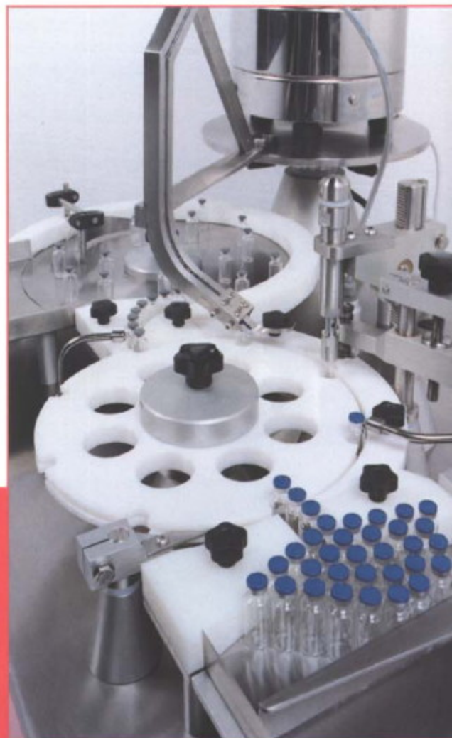
▼ Bambino A with special crimping knife.
