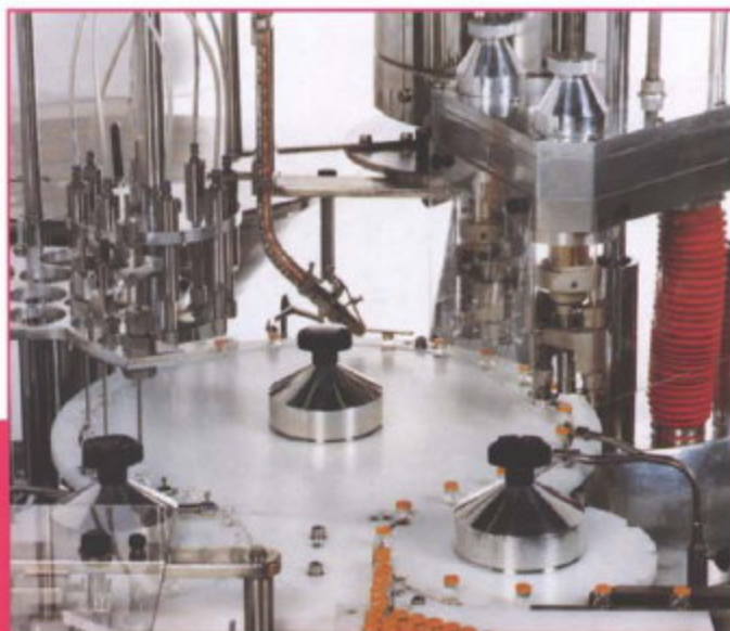
▲ Fill, stoppering and crimping on the same machine.
