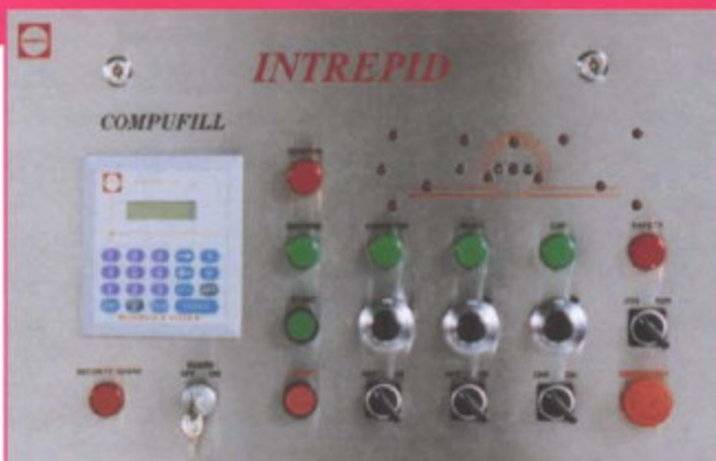
◀ Compufill panel control
