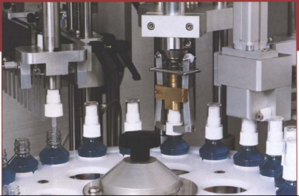
▼ Pump inserter with special cap tightener and overcap station.
