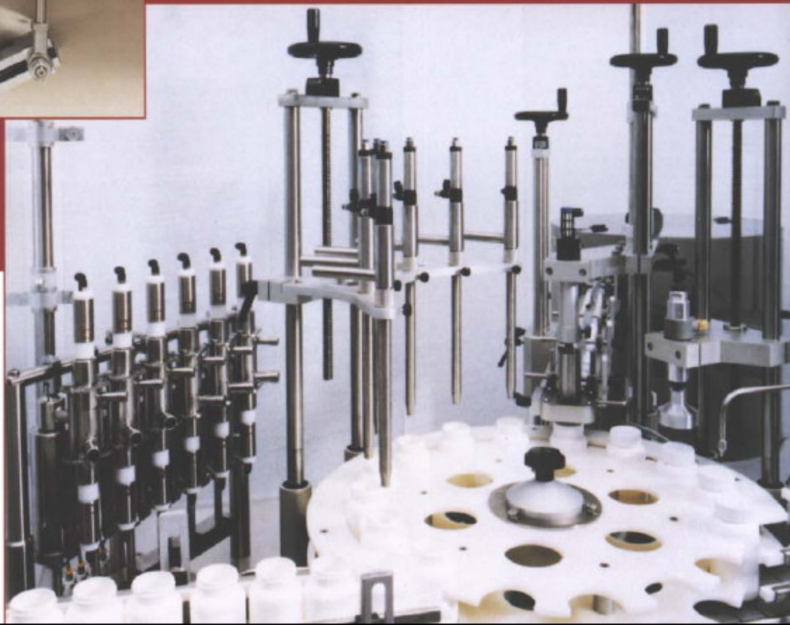
6 Station Compufill system with pretightening cap placement and torquing station. ▼
