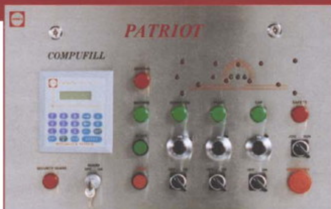
◀ Compufill panel control
