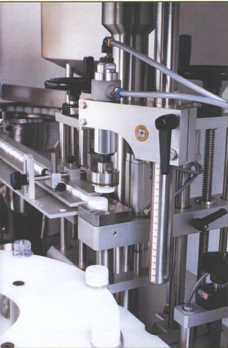
▲ Basic SuperJolly with pick and place capping system and neck support starwheel.
