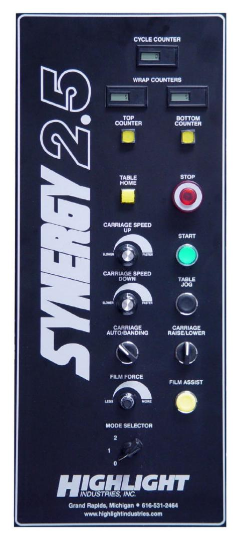
CYCLE COUNTER records number of loads wrapped and assists in scheduling maintenance. Optional resettable cycle counter available.
