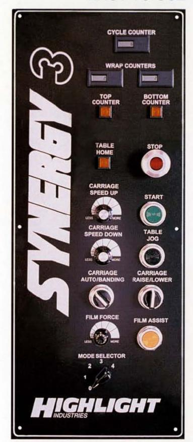
CYCLE COUNTER records number of loads wrapped and assists in scheduling maintenance. Optional resettable cycle counter available.
