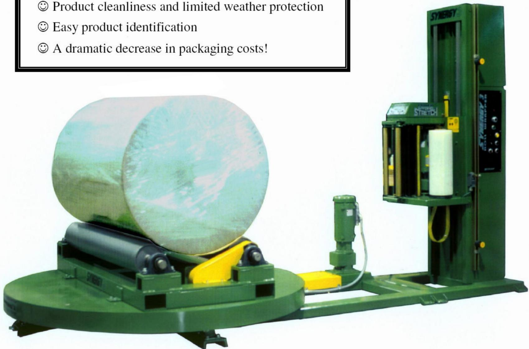
Highlight manufactures the most complete line of roll wrapping systems in the world in addition to the Synergy turntable model shown. Highlight custom designs Freedom™ spiral overhead, Revolver horizontal, and face roll-wrapping machines. Highlight roll wrapping systems are available for small, medium and large rolls with weight capacities up to 25,000 pounds. Highlight Industries is also a leader in the semiautomatic / automatic pallet wrap and stretch bundling machine industry.
